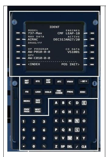
The initial FMC page Looking at the display, we see the aircraft model and engine info, the current NAV DATA cycle and effective dates, and the FMC software version. LSK 6 on the right side (6R), will take us to the POS INIT page when pushed – go ahead and push it now.
